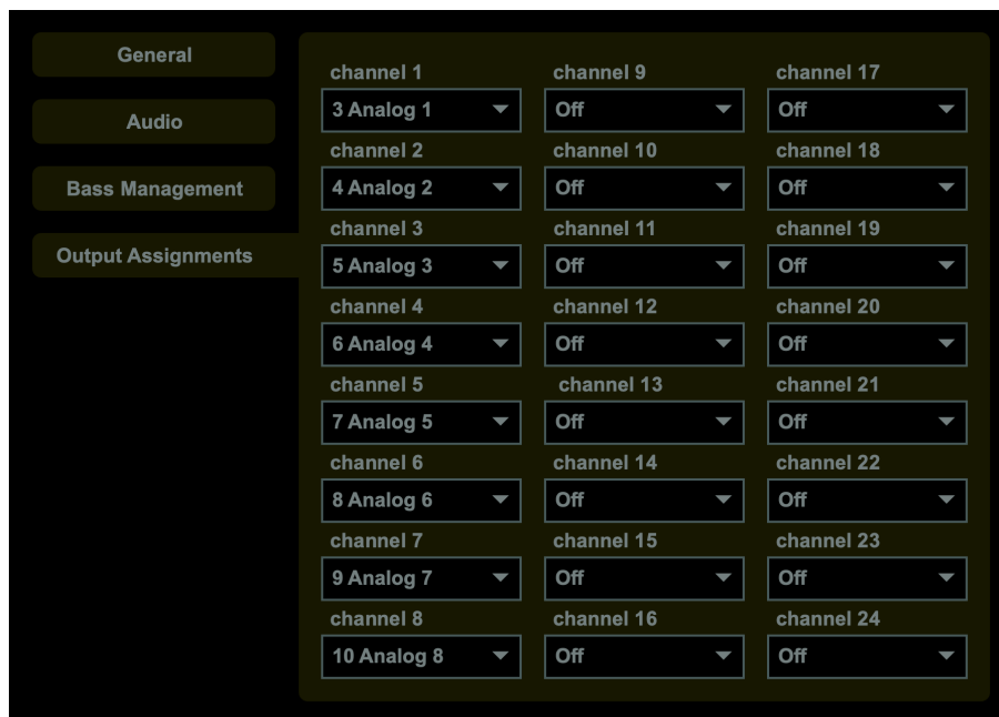
The Output Assignments page of the Preferences window, displaying the routings used in Studio Varèse at UCSB.
